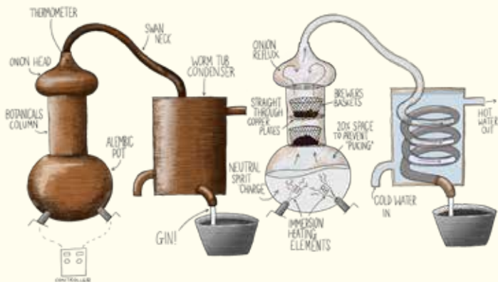
Diagram showing our traditional method for making gin in our copper still 'Ebor'. The herb-infused sugar syrup is added to the distilled gin to produce our Old Tom.
